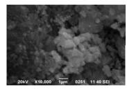
**Figure 2.** SEM image and energy dispersive X-ray microanalysis of "spent" Cu -  $Cr/\gamma$ -alumina catalyst.
