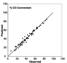
adjustable parameter was the binding energy of H\*. The figure shows a parity plot, with BE of H\* being 262 kJ/mol. The fit is excellent over a wide range of experimental conditions and conversions.
