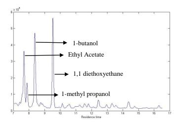
Figure 1. GC-FID Chromatogram of ethanol reaction on Titania in batch reactor. The signal strength is show on the y axis and Residence time on the X Axis. The peaks are labeled. Butanol and 1-methyl propanol can be observed. Unreacted ethanol is not shown. (Conditions of the reaction are 350  $^{\circ}$ C, Pressure =1atm, Catalyst = Titania (8-10 mesh) of 1 g. Ethanol=20 g)
