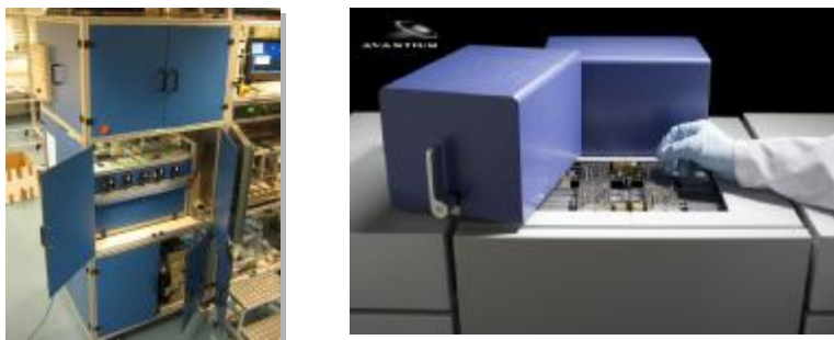
Figure 1: Avantium's Parallel fixed bed reactor systems
