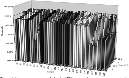
The activity measurements made by the HTS system demonstrate the possibility to identify the most active catalysts from a large number of samples, making it a powerful tool for catalyst development.
